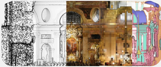
Different renderings of a point cloud. From left to right, raw point cloud, shaded, colored, voxelized, semantized
